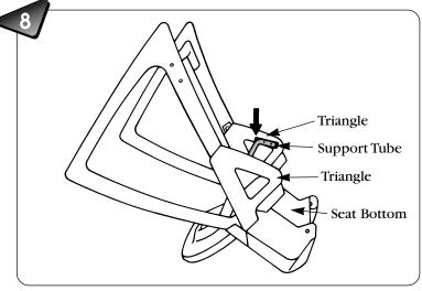
• Push the support tube and triangles all the way down to the seat bottom.
