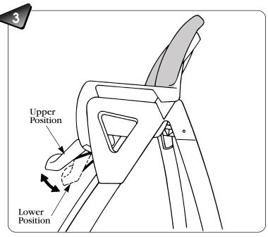
• The footrest can be adjusted to an upper or lower position.
