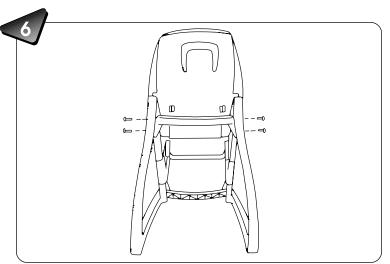
• Insert two 1<sup>1</sup>/<sub>2</sub>" screws into each leg and tighten with a Phillips screwdriver. Do not over-tighten.
