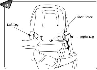
• Fit the back brace between the left and right legs.
