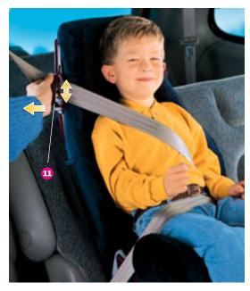
Pull the adjustable shoulder belt positioner out slightly and move it up or down to position the vehicle shoulder belt over your child's shoulder.
