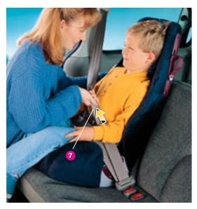
7 Tighten the lap portion of the vehicle lap and shoulder belt by pulling on the shoulder belt.
