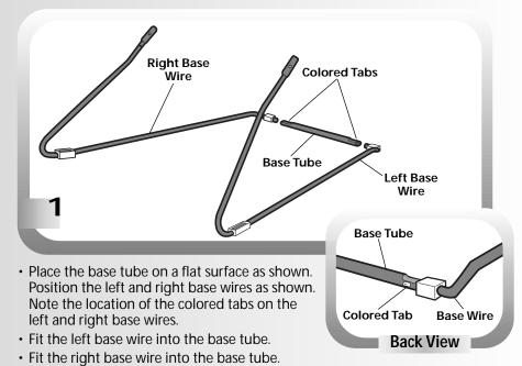
Make sure both colored tabs on the base wires are visible through the holes in the base tube.
