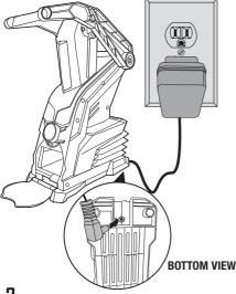
**Note to Adults:** Periodically examine this transformer for damage to the cord, housing or other parts that may result in the risk of fire, electric shock or injury. If the transformer is damaged, do not use it.
