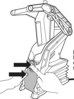
Note: Car mold MUST be inserted correctly before the door will lock.
