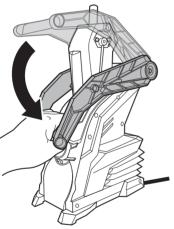
10. When cooldown cycle is complete, the door will unlock. Pull door open.
