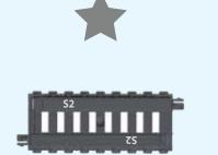
• **ONE-TIME SNAPS**: Assembly steps that are marked with a star are "one-time snaps". Once these parts are put together, they cannot be taken apart.
