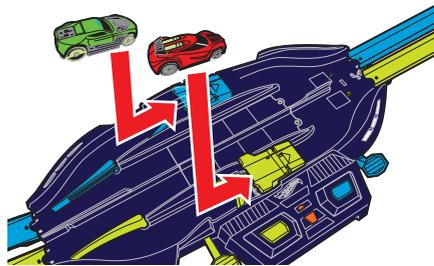
**NOTE:** A FULLY CHARGED CAR SHOULD LAST AROUND 10-15 LAPS. NUMBER OF LAPS WILL VARY DEPENDING ON THE PIT LANE'S BATTERY LEVEL.
