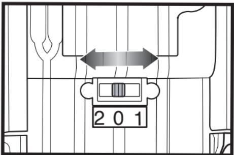
**1 - NORMAL / TEST MODE** (select this mode to test fuel performance)
