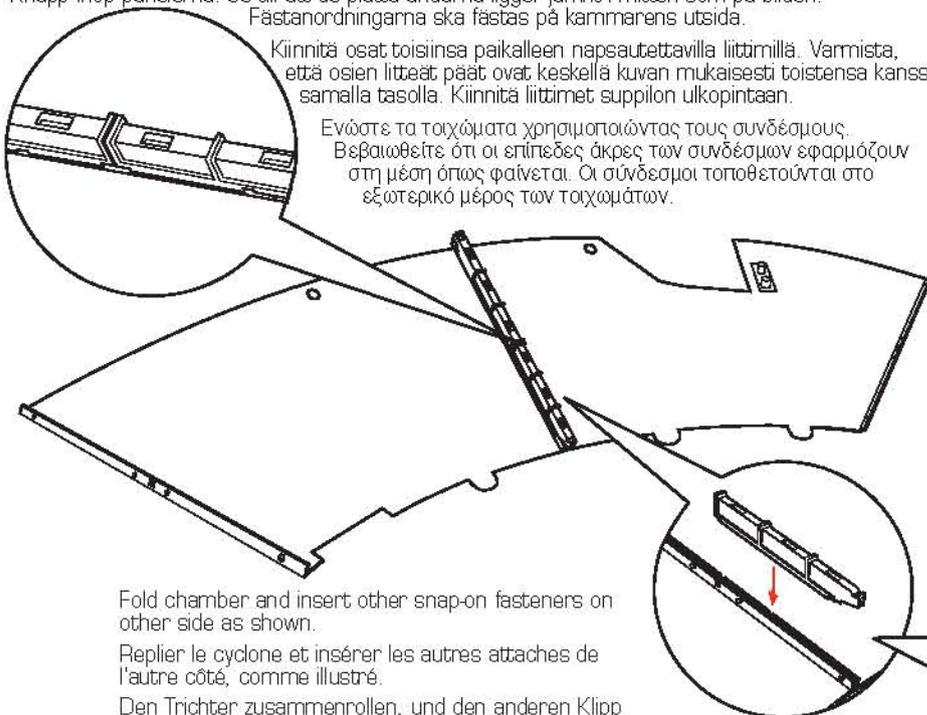
Fold chamber and insert other snap-on fasteners on other side as shown.
