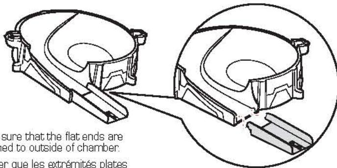
**2.** Connect panels together using snap-on fasteners. Make sure that the flat ends are flush in the middle as shown. Fasteners should be attached to outside of chamber.
