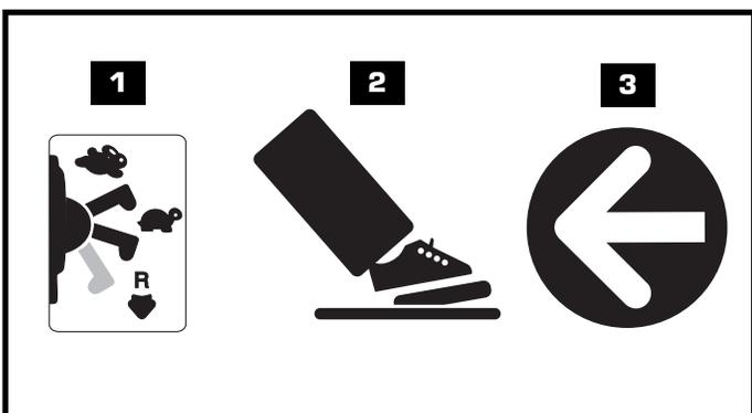
**IMPORTANT!** To avoid damaging the motors and gears, stop the vehicle before shifting from forward to reverse
