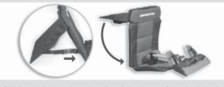
Unfold the seat base and turn the adjust dial at the top of the wheel tripod anti clockwise to loosen the top pivot.
