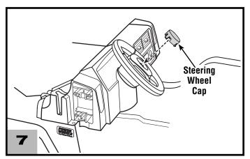
• Insert and "snap" the steering wheel cap into the center of the steering wheel.
