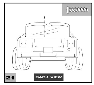
• Insert a #10 x <sup>3</sup>/<sub>4</sub>" screw into the rear edge of the seat. Tighten the screw.
