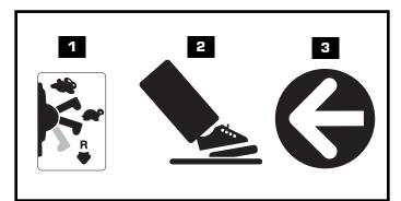
**IMPORTANT!** To avoid damaging the motors and gears, stop the vehicle before shifting from forward to reverse  $\clubsuit$ .
