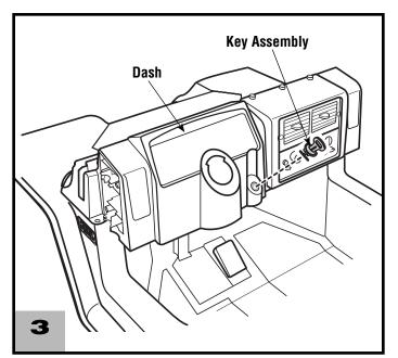
• Insert and "**snap**" the key assembly into the opening in the dash, as shown.
