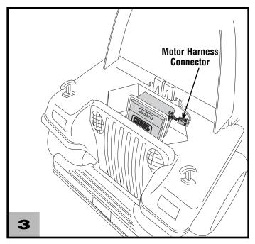
• Plug the motor harness connector into the battery.
