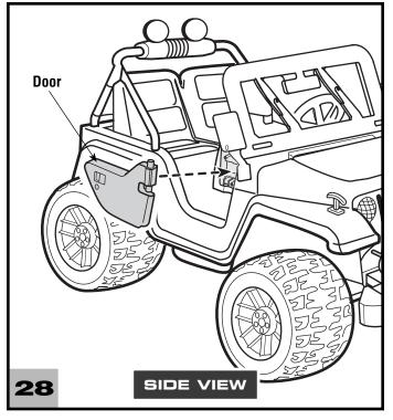
• Fit a door into the groove on the side of the dash. *Hint:* Each door is designed to fit one way. If the door does not fit, try the other door.
