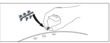
Fix the 6 rubber feet into the holes on the bottom of the Timer as shown.
