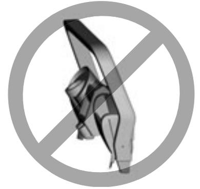
The windshield is **not properly** assembled. Remove the windshield and turn it around so that it bends forward.
