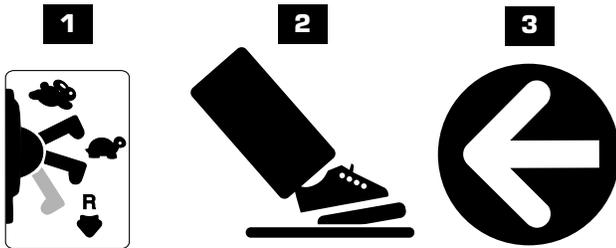
**IMPORTANT!** To avoid damaging the motors and gears, stop the vehicle before shifting from forward to reverse.
