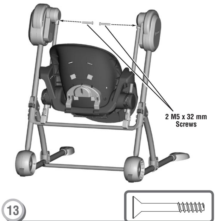
**Note:** Do not attach the seat tubes to the frame crossbar in this assembly step.
