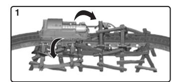
Reset the guard rails by placing them back in the upright position.
