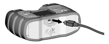
Unplug the USB cord from your computer, then your camera. Slide the power/mode switch off O.
