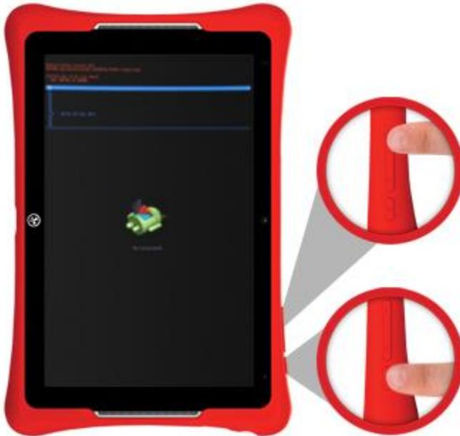
5. When the data wipe is complete, "Reboot system now" should be highlighted. Press the Power button to reboot the nabi Elev-8.
