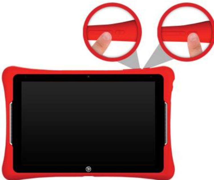
3. Release both buttons and on the "Android System Recovery" menu, use the Volume - button to highlight "Wipe Data/Factory Reset". Then, press the Power button to select that.
