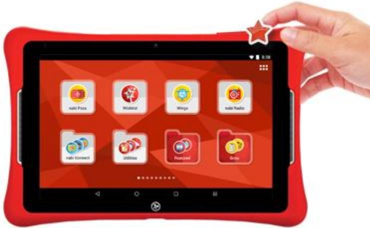
2. Press and hold the Volume + button. Then press and hold the Power button as well until the system menu appears in the upper left corner of the screen.
